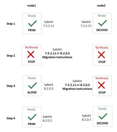
At step 3, check that the module and the application are operationals on node1 before upgrading node2. If not, do not migrate node2 and on node1, rollback to the previous version:
