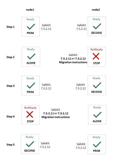
At step 3 (and 4), check that the module (and the application) are operationals on node2 before upgrading node1. If not, do not migrate node1 and on node2, rollback to the previous version:
